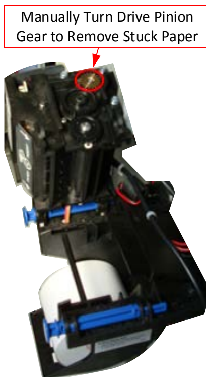
Figure 33. Manually Removing Stuck Receipt Paper
