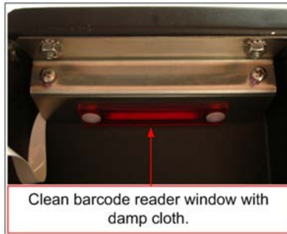
Figure 42. Cleaning the Barcode Reader Window
