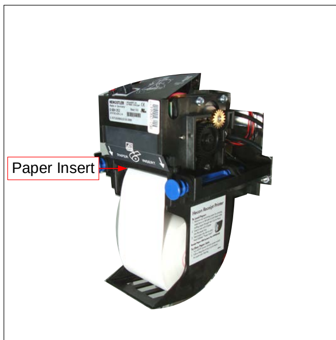
Figure 30. Paper Roll Properly Loaded
