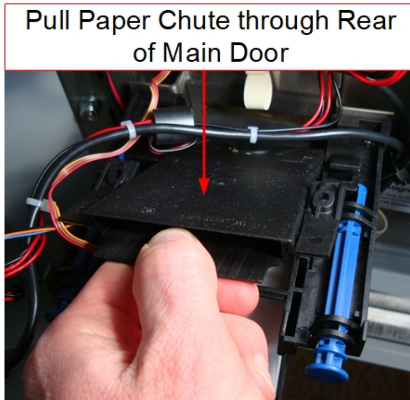
Figure 36. Removing Paper Chute
