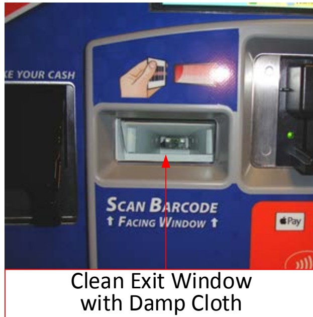
Figure 46. Cleaning Barcode Imager Exit Window
