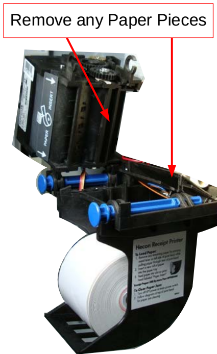
Figure 32. Removing Jammed Receipt Paper
